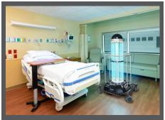
The Tru-D Smart Ultraviolet (UV-C) robot in action. Photo credit: Tru-D® SmartUVC.
